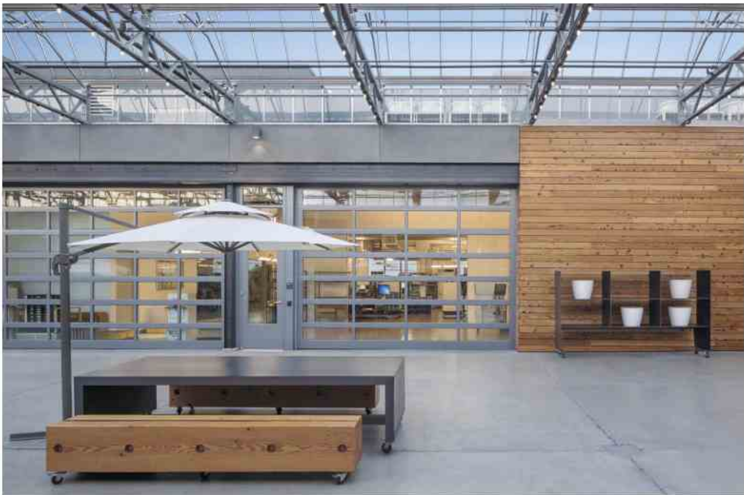
GOOD BONES Original wood roof sheathing, removed to create the atrium, now clads this space's walls (above). The two-story office building was opened up to pay homage to the adjacent warehouse, with exposed wood roof decking and both board-formed and existing concrete elements (left and opposite).
